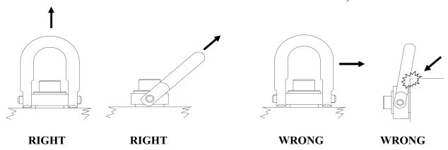
**Important**: The load on each hoist ring is not simply total weight divided by the number of hoist rings. The resultant force can be significantly greater at shallow lift angles and with unevenly distributed loads. See the example and chart below.
