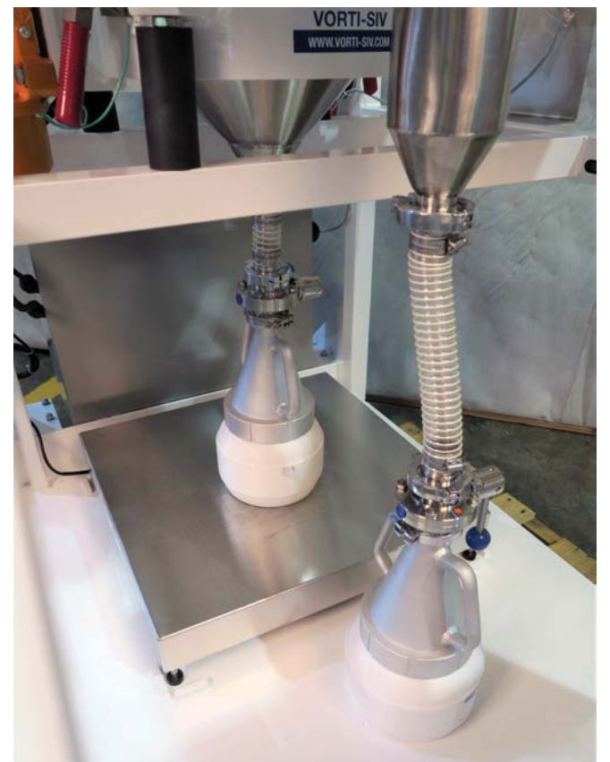
Vac-U-Max on-board sieve and scale separate and weigh reusable powders into industry-standard pail. Oversize/waste debris is also collected (right).
