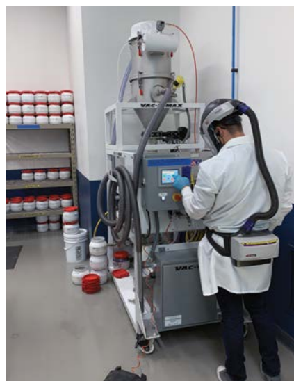
User-friendly HMI control panel with program for continuous conveying, sieving, and weighing of reactive and non-reactive metal powders. Also suitable for ceramic and polymer powders.
