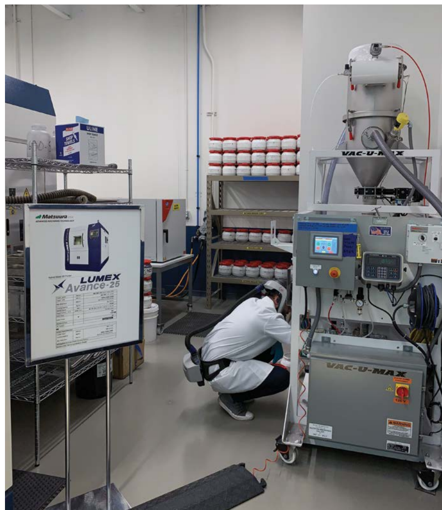
Mobility of the Vac-U-Max MPRS supports multi-printer facilities. The self-contained system includes UL-certified controls and grounding interlock system protects users and their facilities.
