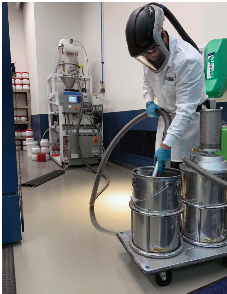
Powered by compressed air or inert gas, the Vac-U-Max MPRS has the suction power to convey metal powders from storage containers 15 ft away for sieving and weighing before re-use.
