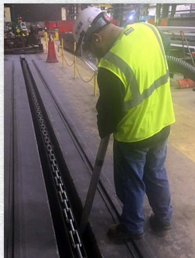
Heavy-duty industrial vacuum cleaners reduce the risk of injuries allowing quick and safe cleaning of heavy materials including steel shot from crevices and other hard-to-reach areas.
