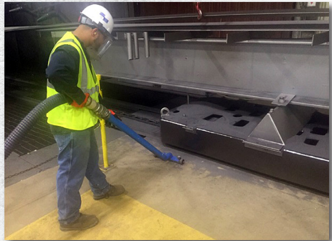
The portable Model 1050 is capable of recovering up to five tons of material per hour including steel shot, and can reduce labor costs by more than 50 percent.
