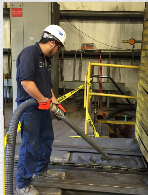
Model 1050 is designed for high volume recovery of many types of materials at rates of 10,000 lbs per hour. As a continuous-duty industrial vacuum cleaner it is the ideal solution to cleanup heavy blast media.
