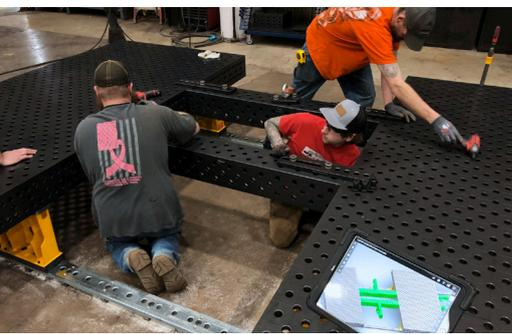
The new Bluco solution was assembled with the help of Bluco engineers using CAD models. It included 5 tables and 12 meters of floor rail.
