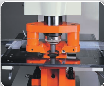
*Urethane spring stripper for minimal deformation.
