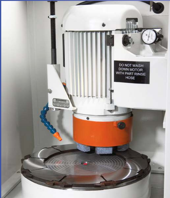
Aircraft brake rotor on 18" magnetic chuck
