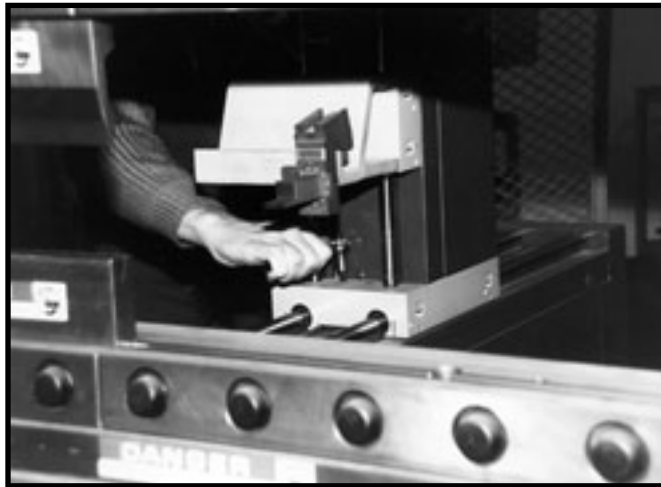
FIGURE 9-22 Loosen X-axis carriage drive bolts
