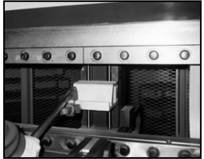
FIGURE 9-30 Z-axis, align center of gage fingers
