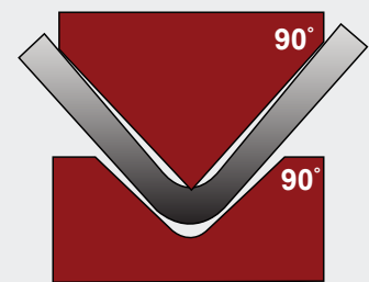
FIGURE 2 - OVERBENDING DURING FORMING OPERATION
